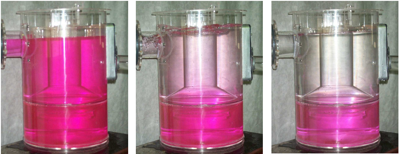
Figure 4 – Dye Tracer Studies Confirming the Ability of the Internal Components in an Advanced Vortex Separator (AVS) to Isolate the Pollutants Storage Region
